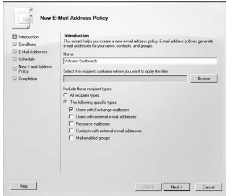
FIGURE 16.7 Naming the email address policy and defining the objects to which it applies
